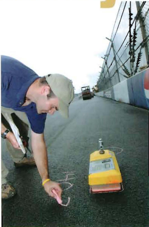
Brian Prowell of NCAT checks the density of paving. NCAT personnel verified mix designs, performed QA testing, and monitored density during construction.
