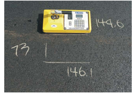
Average mat density reached 94.7 percent and average joint density while paving in echelon was 94.1 percent; the target density was 94. Photo credit: Advanced Material Services LLC
