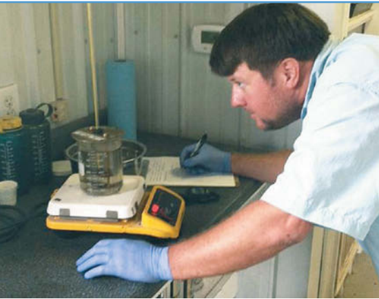
A binder softening point of 180°F was specified and confirmed for every tanker of binder delivered to the project. Photo credit: Advanced Material Services LLC
