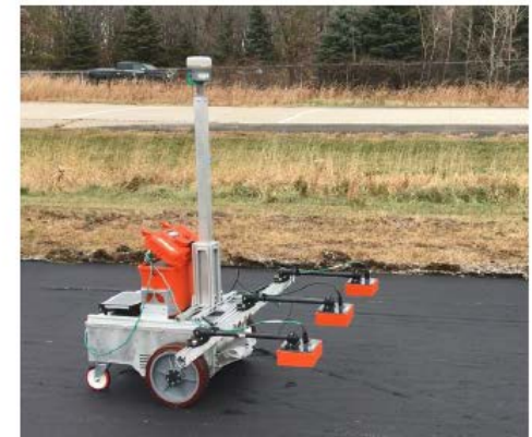
Figure 1.1. LEFT-Integrated Robot; RIGHT-integrated GPR system shows mounted GPR sensor array and data acquisition system during field test on fresh asphalt.
