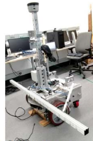
Figure 1.1. LEFT-Integrated Robot; RIGHT-integrated GPR system shows mounted GPR sensor array and data acquisition system during field test on fresh asphalt.
