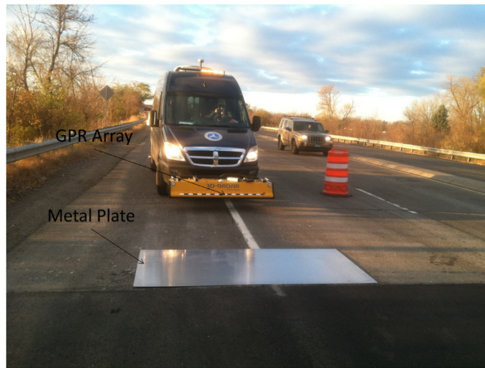
Fig. 1. Illustration of the vehicle mounted step frequency array system.
